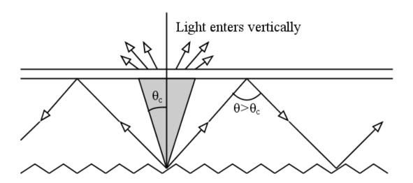
All light reflected within the Lambertia cone with an angle equal to the critical angle for total internal reflection can exit the Si. All other light is 'trapped' through total internal reflection Back surface roughened to randomize direction of reflection from back surface
