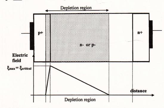
The Punch-through (PT) high voltage diode is a based on a PIN diode where the thickness (length) of the lowly doped layer (n- or p-) is smaller than the depletion region thickness (length) at breakdown. Thus the depletion region reaches the n+ cathode region before avalanche breakdown takes place.
