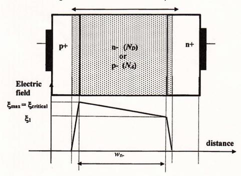
For the BJT the PT design is more appropriate. The drift length is shorter in the PT design, and since the BJT operates in hard saturation, the charge in the drift region (collector) is much greater than the doping, so a PT design will ensure minimum drop across this region. [40%]
