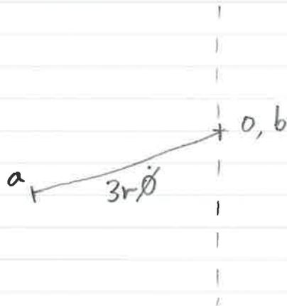
$$\omega_{AB} = \frac{ab}{AB} = \frac{3r\dot{\phi}}{3r} = \dot{\phi} \quad \text{clockwise}$$
