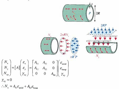
The transformed stiffness matrix for the ±60° plies is given by
