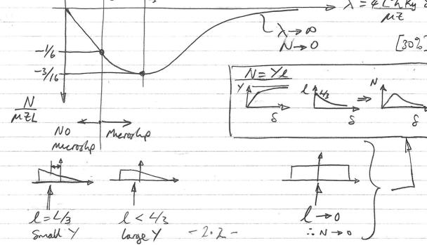
look (d) Realigning moment is usually reglected in simple models of vehicle dynamics because the preumatic trail is small relative to length of the vehicle, ie N is small relative to yourne moments on the vehicle body due to Y.
