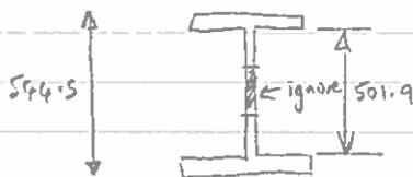
$$\therefore \text{Reduce area by } (0.2 \times 501.9) \times 12.7 = 1275 \text{ mm}^2$$
