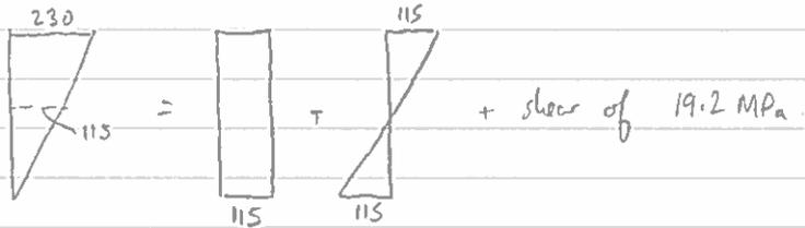
$$\sigma_c = 115 \text{ MPa}, \quad \lambda = \frac{488}{12} \sqrt{\frac{275}{355}} = 35.8 \geq 24 \therefore \text{Not compact in compression}$$
