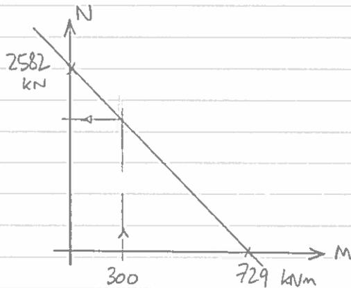
$$N_{\text{max}} = 2582 - 2582 \left( \frac{300}{729} \right) = \underline{\underline{1519 \text{ kN}}}$$
