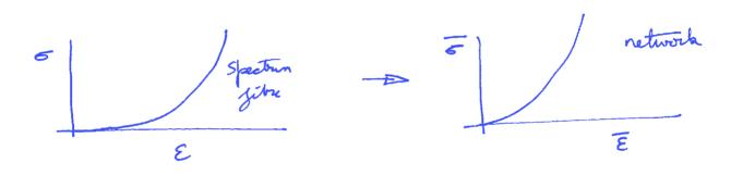
when the files are pulled strought they have a high modulus & strength
