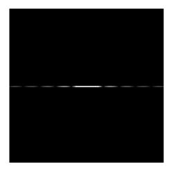
Note that the pixel wide strip is in fact shifted to the right by a distance d. This will not effect the intensity of the plot above but it will add a phase term in the Fourier plane.
