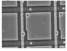
Above we assumed that the pixel pitch matched the finite width of the pixels themselves. This is not the case in reality as each pixel must have a gap between itself and its neighbour to prevent short circuits and to allow for transistors etc to be used to drive the pixels. This region between the pixels is referred to as the deadspace and the ratio of pixel size to pixel pitch is called the fill factor.
