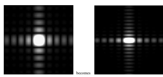
As we extend the pixel in the vertical direction, we will shrink the width of the sinc function in the v dimension of the replay field. Note that the u dimension does not change and remains as the fundamental sinc function. Eventually the single pixel will ne extended to a long thin vertical strip of width  $\Delta$  as shown in Figure 1(a). If the strip is infinitely long, then the v dimension in the replay field becomes infinitely thin (in its limit a delta function.
