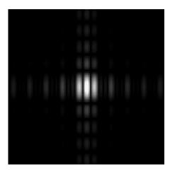
The same principle as in part (a) applies. As we add more shifted pixels, the width of the resulting sinc function decreases and ends up as a series of delta functions that have the same odd harmonic structure and have an envelope given by the original single pixel sinc function. If the shifted pixels are in fact the pixel wide strips shown in Figure 1(a), then the periodic structure in the replay field will be made from delta functions in both the u and the v dimensions.
