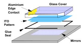
The use of the Si backplane means that the power of electronics can be i=used to interface with the SLM. This allow pixel arrays with very small pitches (<5um) and also allows them to be addressed at high speeds. Other features such as processing, demultiplexing and compression can be added to the electronics on the backplane.
