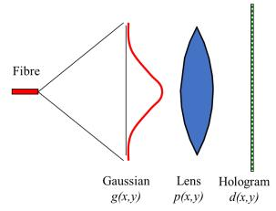
The entire illumination system can be modeled as a sequence of multiplied functions. The input illumination distribution g(x,y) times the hologram aperture d(x,y) times the total aperture of the FT lens (if it has a smaller diameter than the hologram) p(x,y). Hence effect of the FT on these functions results in a convolution of their transforms.
