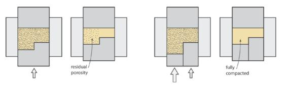
(b) Assume that there is no flow of material between the two parts of the die, so compaction occurs uniaxially in each half, i.e. the volume of solid is separately conserved in each half, and the same vertical strain is applied.
