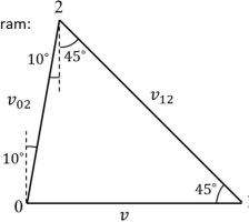
Relative velocity, workpiece vs chip:  $\frac{v_{12}}{\sin 80^\circ} = \frac{v}{\sin 55^\circ}$ ,  $v_{12} = 1.202v$
