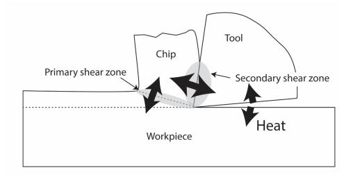
In machining processes, the temperature rise is a critical aspect due to the intense plastic deformation and friction involved. The temperature rise occurs primarily in two key zones:
