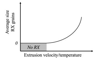
smaller average grain size (locally). See the relationship between strain and grain size in  $R\boldsymbol{X}$
