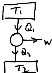
Clausius (applied to engine as the system)  $\Rightarrow \frac{Q_1}{T_1} - \frac{Q_2}{T_2} \leq 0$
