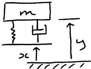
$$\begin{aligned} m\ddot{x} &= \lambda(s_c - y) + k(x - y) \\ m\ddot{x} + \lambda\dot{y} + ky &= \lambda s_c + kx \\ \Rightarrow \text{case } (c) \end{aligned}$$
