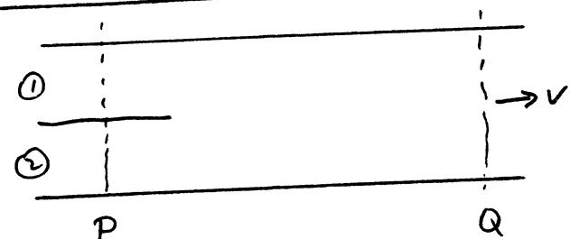
S.F.E.E. applied to pipe between P & Q ( $\dot{Q} = \dot{w}_x = 0$ )
