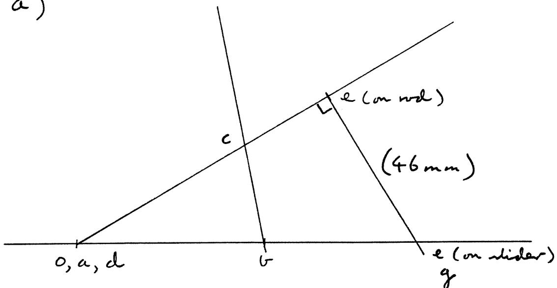
From diagram, velocity of  $G = \underline{91} \text{ mm/s}$
