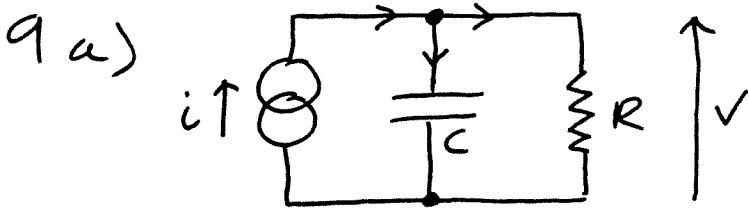
$$i = C \frac{dV}{dt} + \frac{V}{R} \quad \text{where } \frac{1}{R} = \left( \frac{1}{200 \times 10^3} + \frac{1}{300 \times 10^3} \right) \rightarrow R = 120 \times 10^3$$
