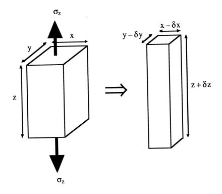
(b) Before deformation : volume  $V_0 = xyz$
