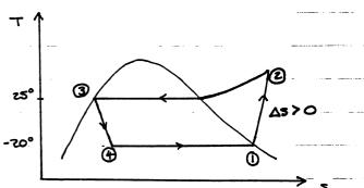
$h_1 = 178.7 \text{ kH/kg}$   $h_2 = 212.1 \text{ kH/kg}$   $h_3 = 59.7 \text{ kH/kg} = h_4$
