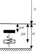
Momentum is conserved through the impact. (c)  $mv_o = 2mv_1$ , where  $v_i$  is velocity after impact  $\Rightarrow v_1 = v_0/2$
