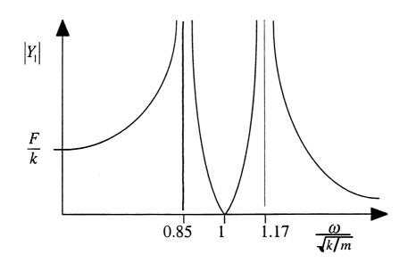
$|Y_1| = 0$  when  $k\alpha = \omega^2 m/10 \Rightarrow \omega \Rightarrow \sqrt{k/m}$  (resonant frequency for added mass)  $|Y_1| = F/k$  for  $\omega \to 0$  (static response)
