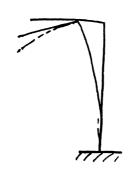
Uc: Horgontal deflection of  $C = h_0 = 0.0078 \, \text{m}$ Uc: Vertical deflection of  $C = \Theta_0 \times 0.25 \, \text{m} + \text{Uc}$   $= 0.0091 \, \text{m}$ Uc: Rotation of  $C = \Theta_0 \times 0.25 \, \text{m} + \text{Uc}$   $= 0.0091 \, \text{m}$   $= \Theta_0 + \Theta_c$   $= 0.0391 \, \text{rad}$
