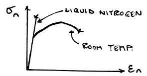
This occurs because slip is more difficult as temperature falls in BCC iron, whereas FCC aluminium is always ductile.
