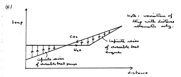
Temperature differences between streams used to drive everyies (or overcome lay beat pumps - as appropriate). Since there is overall enthalpy balance, no net shaft work and everyines just drive pumps. BUT result may be only truefer of universitably to test source
