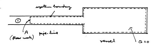
consider as system all the H2O contained in the versel at the line of viterant in the changing process, when the state is denoted (2). I wittelly the system (mars m) was in the page line at state (3).
