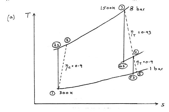
(ii) Since work output of h.p. turbine drives the compressor,
