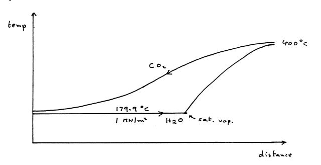
Since we overall feat transfer between evelouser and summarish and no shaft work, SFEE given evillally drop of  $Co_2$  = enthalpy vie of  $H_2O$ , with sp. At. especitly of  $Co_2$  = 0.82 (lable 2) and wetlet temp of  $Co_2$  = 179.9°C, man of  $Co_2$  pr ty  $H_2O$  given by  $M_{co_2} = 0.82$  (400 - 179.9) = 1 (3264 - 762.6)
