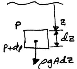
b) PRESSURE ACTS EQUALLY IN ALL DIRECTIONS. HENCE PRESSURE FORCE IS PERPENDICULAR TO SURFACE AND SURFACE IS FLAT.
