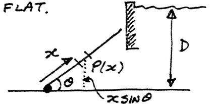
[ALT: COULD USE NET HORIZONTAL FORCE, OR JUSTIFY LINEAR PRESSURE VARIATION AND STATE AVERAGE PRESSURE  $\times$  AREA.]
