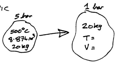
MASS REMAINS IN CYL :  $M_{LEFT} = \frac{P V_{CY}}{RT} = \frac{1 \times 10^5 \times 8.874}{287 \times 488.1} = 6.335 kg$
