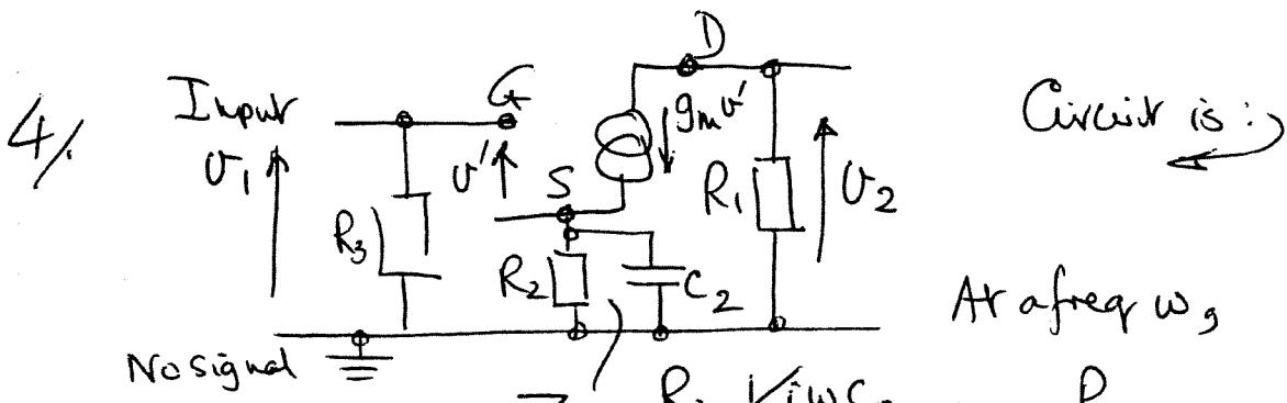
$$Z = \frac{R_2 \cdot 1/j\omega C_2}{R_2 + 1/j\omega C_2} = \frac{R_2}{1 + j\omega C_2 R_2}$$
