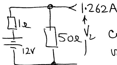
With the Ammeter replaced, the circuit becomes as shown. The new voltage  $V_2$  across the circuit given by
