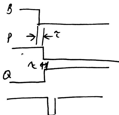
Fix hazard by adding an extra gate A.C to g. the circuit so that there is one big "a" k-map.
