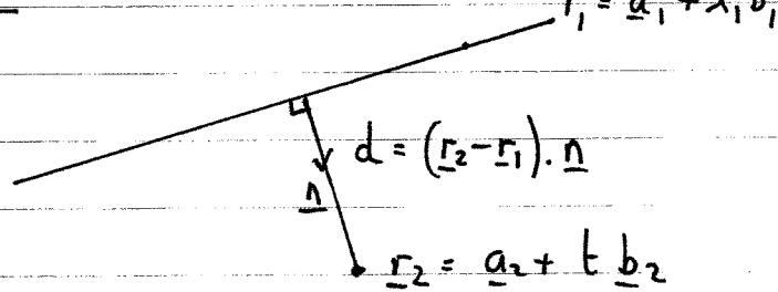
Perpendicular distance is  $d = \left| (\underline{a}_2 - \underline{a}_1) \cdot \underline{n} \right|$
