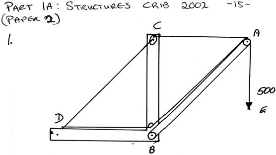
Main lifting cable must carry 500 KW huffing cable must also carry 500 KW (by taking moments about B).
