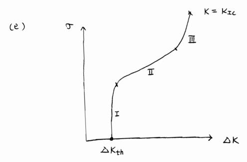
If  $\Delta K < \Delta K$ th, no crack growth is detected. When the crack has grown sufficiently long such that  $K = K_{IC}$ , fast fracture occurs.
