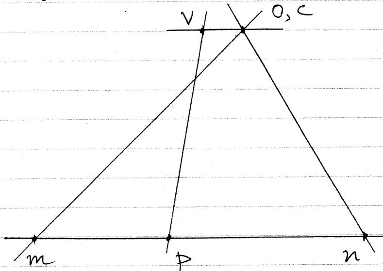
Note that  $\frac{pm}{nm} = \frac{PM}{NM} = \frac{40}{100} = \frac{pm}{90 \text{ mm diagram}}$
