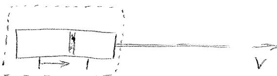
$$F = \rho A v^2 = 10^3 \times 2 \times 10^{-6} \times 40^2 = 3.2 \text{ N} \quad \text{initially}$$
