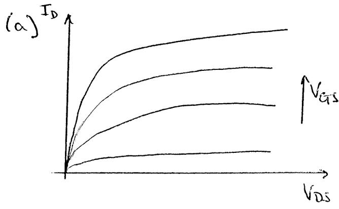
From the FET's output characteristic, we can estimate  $\frac{\partial I_D}{\partial V_{GS}}$  (slope of the lines in the linear region) and  $\frac{\partial I_D}{\partial V_{DS}}$  (spacing of the lines in the linear region). For variations, simple mathematics tells us that
