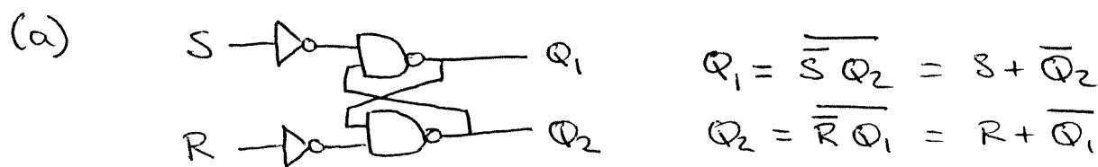
For useful operation, avoid  $S=R=1$ .  $S=1, R=0$  turns on  $Q_1$ , off  $Q_2$ .  $S=0, R=1$  turns on  $Q_2$ , off  $Q_1$ .  $S=R=0$  leaves outputs as they are.
