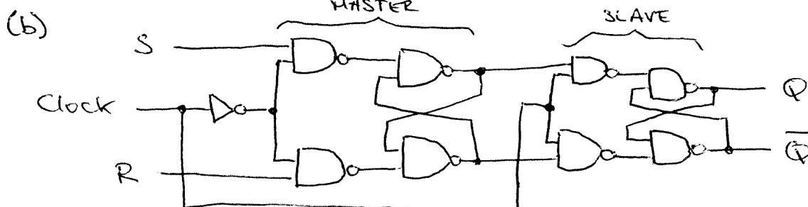
When the clock is low, the master bistable is sensitive to the S-R inputs, while the slave outputs remain as they are. As the clock rises, the state of the master bistable is transferred to the slave. It is still necessary to avoid  $S=R=1$ .
