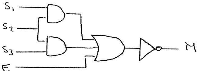
$$(c)(i) M = \overline{E} \overline{S}_2 + \overline{E} \overline{S}_1 \overline{S}_3 = \overline{\overline{E} \overline{S}_2} \cdot \overline{\overline{E} \overline{S}_1 \overline{S}_3} \quad - \text{i.e. 3 NAND gates}$$
