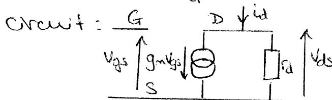
The use of the equivalent circuit greatly facilitates the small signal analysis of FET circuits (gain, input/output impedance etc...)
