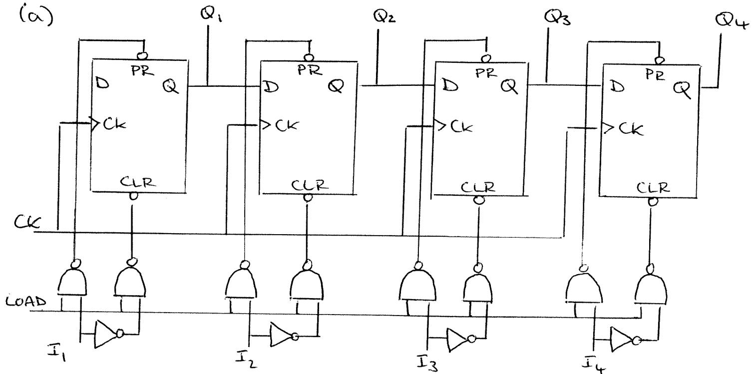
When the LOAD line goes high, the data on the parallel inputs  $I_1, \dots, I_4$  is loaded into the four D-type flip flops. On the rising edge of each clock (CK) pulse, the data is shifted one place to the right, so it all eventually appears, serially, at output  $Q_4$ . The circuit therefore functions as a parallel to serial converter.
