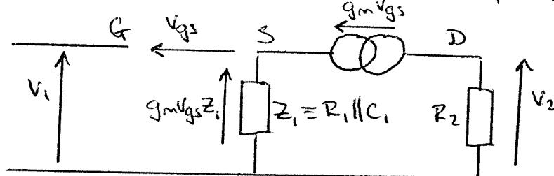
(c) (i) From diagram,  $V_2 = -g_m V_{GS} R_2$  and  $V_1 = g_m V_{GS} Z_1 + V_{GS}$
