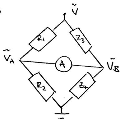
$$\bar{V}_A = \frac{R_2 \bar{V}}{R_1 + R_2} \quad \bar{V}_B = \frac{Z_4 \bar{V}}{Z_3 + Z_4}$$
