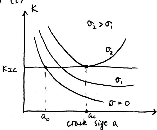
This plot shows the influence of applied stress  $\sigma$  on growth of an arrested indentation crack, length  $a_0$ . The additional term in  $K$  leads to a minimum in the total  $K$ , corresponding to a crack length of  $a_c$ . The crack undergoes stable growth as  $\sigma$  is increased. Once  $a = a_c$ , the condition for final (unstable) failure is obtained.
