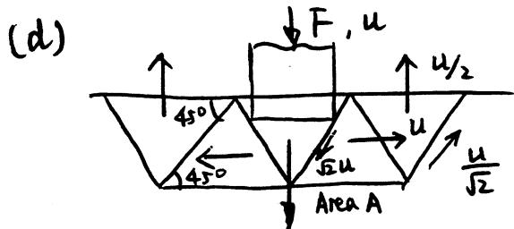
$$\begin{aligned} \text{Net work done} &= Fu \\ &= \frac{2kA}{\sqrt{2}} u\sqrt{2} + 2Ak u + 4k \frac{A}{\sqrt{2}} \cdot \frac{u}{\sqrt{2}} \\ &= 6Ak u \Rightarrow F = 6Ak \end{aligned}$$
