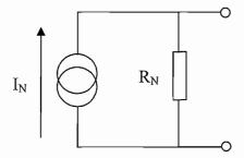
where  $I_N = I_{SC}$  and  $R_N = V_{OC}/I_{SC}$
