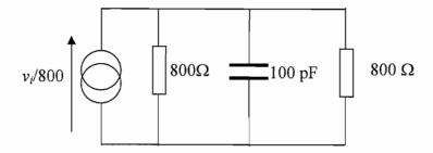
The two 800  $\Omega$  resistors may be combined in parallel to give 400  $\Omega$ . Denoting R = 400 $\Omega$  and C = 100 pF the capacitor voltage,  $v_c$ , is:
