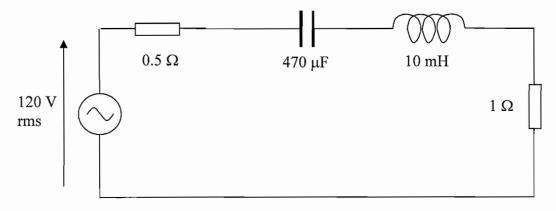
ii) Resonant frequency  $\omega_0 = 1/\sqrt{LC}$  and  $f_0 = \omega_0/2\pi$  giving 73.4 Hz
