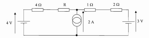
Now convert right-hand side to Norton to give a 1 A current source in parallel with a 3  $\Omega$  resistor, and combine this 1 A current source with the 2 A current source by adding (since they are in parallel):
