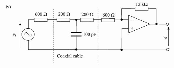
The mid-band voltage gain assumes that  $\omega$  is low enough so that the 100 pF capacitor is an open-circuit. In this case all the series resistors in the circuit above may be lumped together to give 1600  $\Omega$ . Using earlier results: Mid-band voltage gain  $v_o/v_i = -12000/1600 = -7.5$
