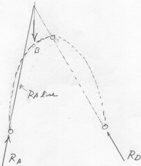
Draw the force diagram like the one shown in the left figure using the scaled figure given in the question. By inspection, the largest separation between section AB and the RA-line is at B (2.0.8). The maximum moment will be at this location.
