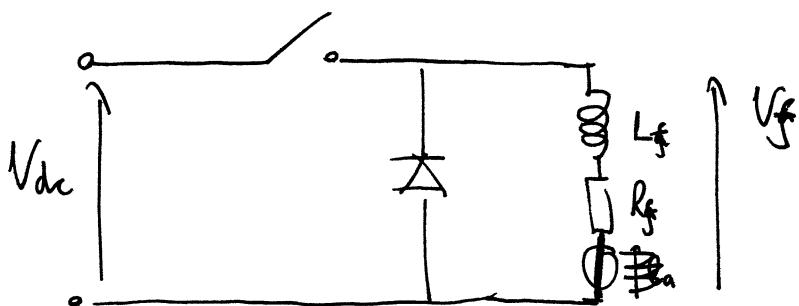
Diode gives free wheel path for armature current to flow in when switch is open, clamping  $V_f$  to 0V. When switch is closed,  $V_f = V_{dc}$ .
