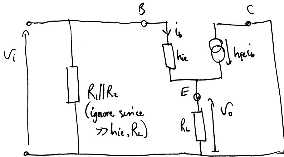
$$V_o = (h_{fe} + 1) i_b R_L$$
