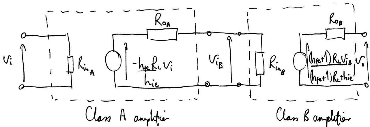
$$V_{i_B} = \frac{R_{i_{inB}}}{R_{i_{inB}} + R_{O_A}} \times \left( -\frac{h_{fe} R_C V_i}{h_{ie}} \right) \quad (\text{Potential divider})$$
