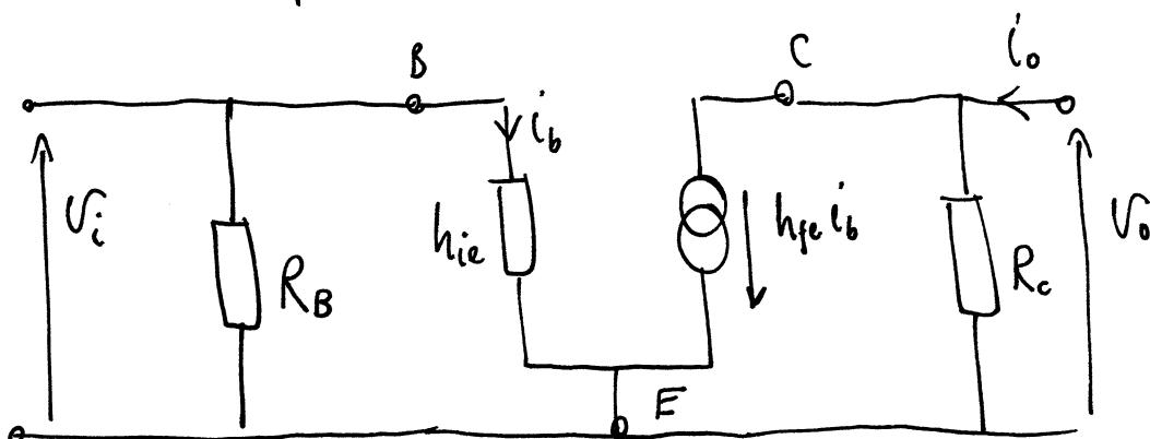
$$i_b = \frac{V_i}{h_{ie}} \quad V_o = -h_{fe} i_b R_c = -h_{fe} \frac{V_i}{h_{ie}} R_c$$
