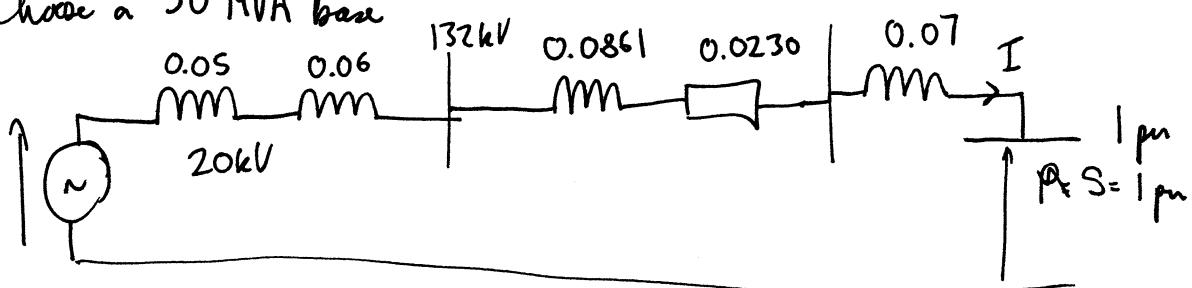
$$\text{For the feeder, } Z_b = \frac{V_b^2}{VA_b} = \frac{(132 \times 10^3)^2}{50 \times 10^6} = 343.5 \Omega$$
