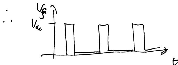
By controlling the mark:space ratio of the chopper, the average field voltage is controlled, and hence the average field current.
