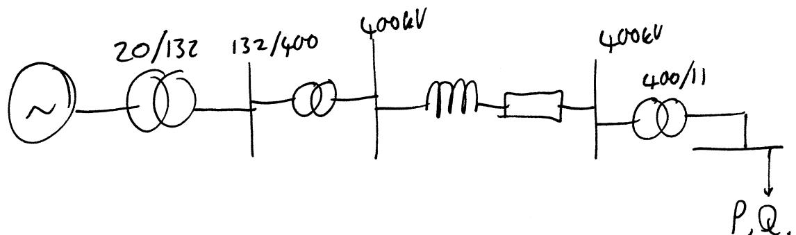
Since the load voltage, power and reactive power remain the same, so will the load current.
