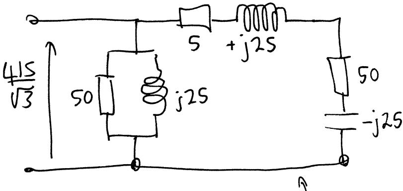
$\therefore$  One phase of this 3 $\varphi$  load looks like, which reduces to
