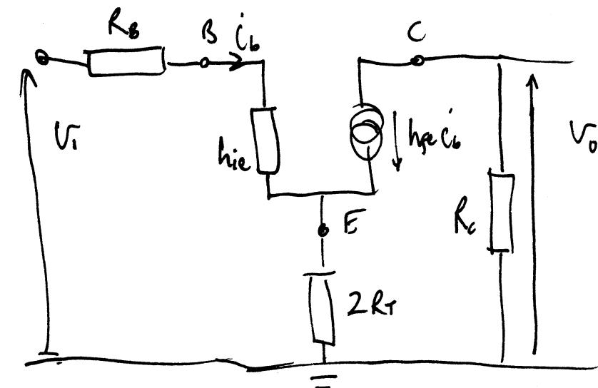
$$V_i = (R_B + h_{ie}) i_B + (h_{fe} + 1) i_B \cdot 2R_T$$
