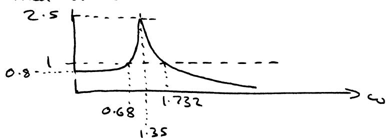
Expect response to be fairly oscillatory (due to large peak in freq response) at a freq of  $\approx 1.35 \text{ rad s}^{-1} = 0.2 \text{ Hz}$
