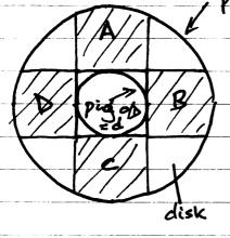
For vertical movement of the pig elements A and C att in tension/compression and elements Band D in show
