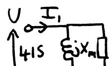
$\frac{3 \times V_1^2}{R_0} = 600 \Rightarrow \frac{3 \times 415^2}{R_0} = 600$
