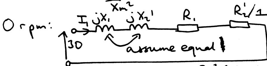
$$3I_1^2(R_1 + R_2') = 333 \Rightarrow \left(\frac{8}{\sqrt{3}}\right)^2(2 + R_2') = 111 \Rightarrow R_2' = 3.2 \Omega$$
