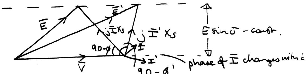
by changing excitation voltage using field regulator, the shape of the diagram changes and so  $\phi$  varies. Hence for constant power  $Q$  varies because of change in p.f.
