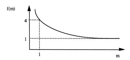
(d) Probability of failure = 50% in bend test for an applied maximum stress (i.e. at the upper surface of the specimen) of 214 MPa. An applied stress of 214 MPa in a bend test, therefore, corresponds to a strength of  $\frac{214 \text{ MPa}}{[2(m+1)]^{1/m}} = 130 \text{ MPa} \text{ in an axial tensile test.}$
