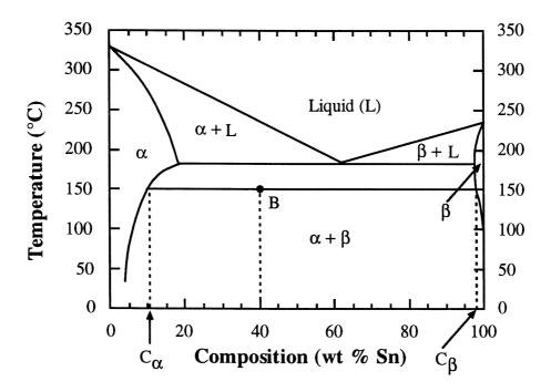
It is necessary to employ the lever rule to determine the relative amount of each phase present in the 40 wt % Sn and 60 wt % Pb alloy in terms of its mass fraction since the
