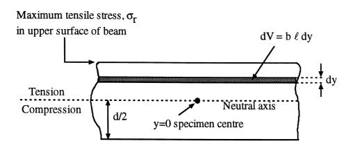
For the specimen in pure bending;
