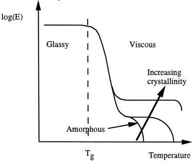
Modulus falls typically by a factor of up to 500 at  $T_g$  and occurs at a temperature of between 0.5 and 0.8  $T_m$ . Depends on degree of crystallinity of polymer, however.
