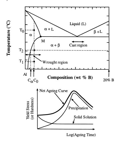
(c) Full marks for a solution which explains; (i) the difference between heat treatable and non heat treatable wrought alloys; (ii) the eutectic nature of cast alloys which generally inhibits the formation of precipitates and hence hardening; (iii) 2 examples.
