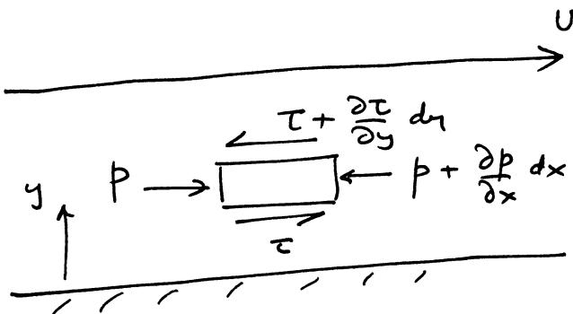
$$\frac{\partial \tau}{\partial y} dy dx = \frac{\partial p}{\partial x} dx dy \quad \therefore \frac{\partial \tau}{\partial y} = \frac{\partial p}{\partial x}$$
