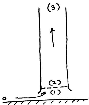
$$\text{Continuity } 1-2, \rho_1 V_1 = \rho_2 V_2$$
