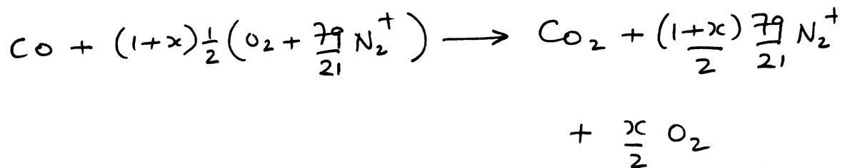
SFEE  $Q = H_{P_2} - H_{R_1} = (H_{P_2} - H_{P_0}) + (H_{P_0} - H_{R_0})$
