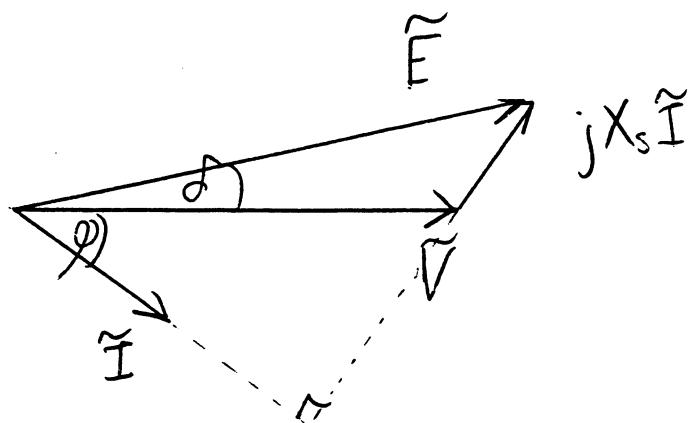
Phasor diagram for a typical operating point when generating has its sides scaled by  $3V/X_s$ :
