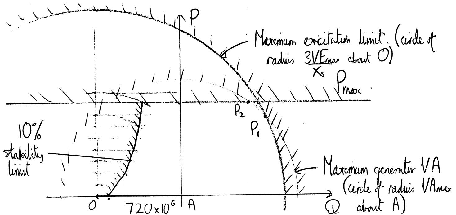
$P_{\max} = 800 \text{ MW} \Rightarrow \text{horizontal line at } 800 \times 10^6 \text{ since } P = 3VI_{co}$
