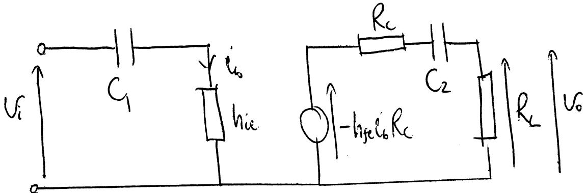
As before, replace  $h_{ie}i_B \parallel R_C$  with  $-h_{fe}i_B R_C$  in series with  $R_C$
