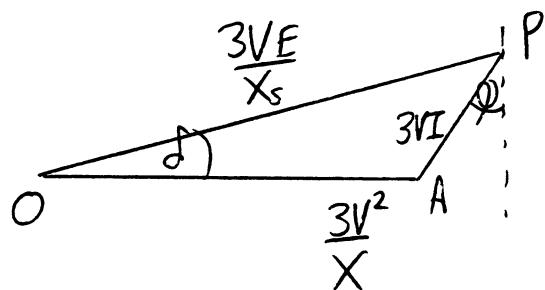
Now the limits on  $P_{max}$ , VA, excitation and stability can all be marked on to give the operating chart.
