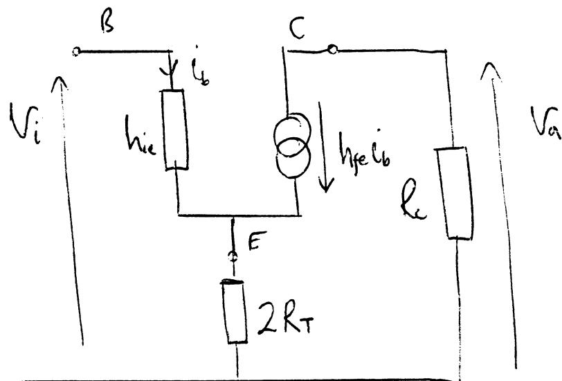
$$V_i = h_{ie} i_b + 2R_T (h_{fe} + 1) i_b$$
