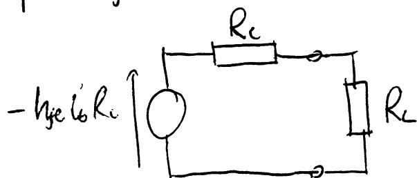
By maximum power transfer theorem  $R_L = R_C$
