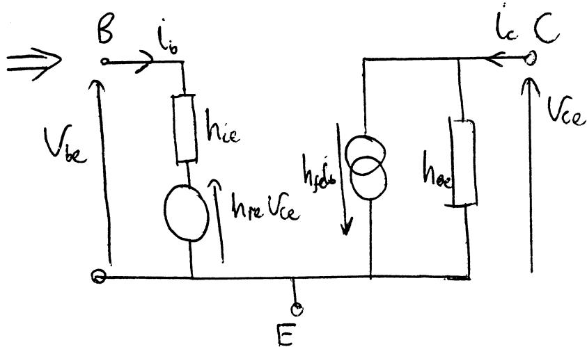
It is seen that the circuit linking C to E represents ①, that linking B to E represents ②
