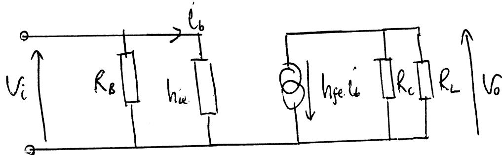
Replace  $h_{FE} i_b / R_C$  with Thvenin equivalent
