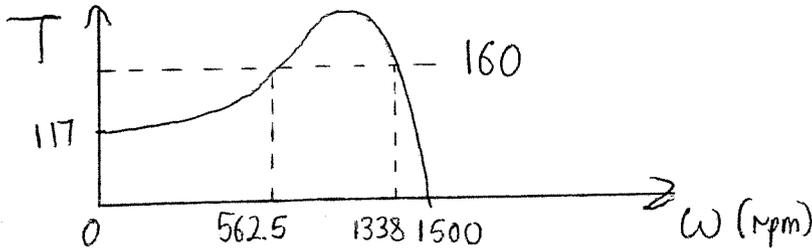
c)  $\eta = 77.5 \%$  at 1338 rpm, 20 % at 562.5 rpm. Therefore, operating at 1338 rpm is preferable. d) Connect additional rotor resistance via slip-rings.
