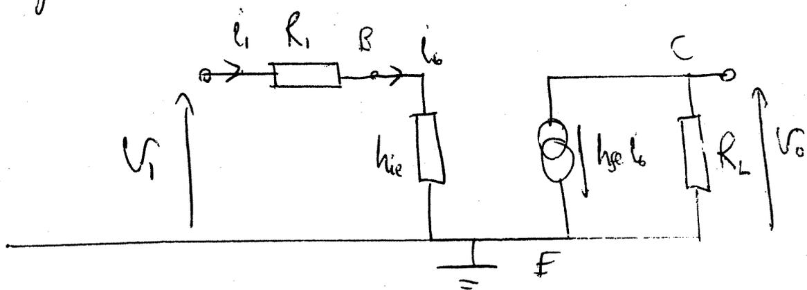
$$i_b = \frac{V_i}{R_1 + h_{ie}} \quad V_o = -h_{fe} i_b R_L = -\frac{h_{fe} V_i R_L}{R_1 + h_{ie}}$$
