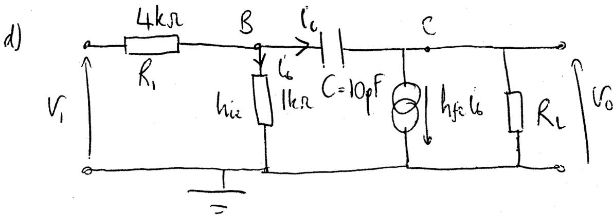
At high frequencies  $\frac{1}{j\omega C}$  is small, and so  $I_b$  is reduced owing to shunting effect of  $C$ . In turn,  $V_o \propto I_b$ , and so gain is reduced.
