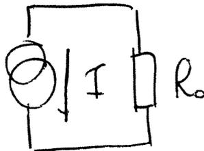
avoids excessive  $V_{EE}$  whilst retaining high effective  $R_T$  and hence CMRR.
