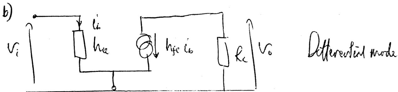
Use half-circuit for differential input, with  $R_T$  a short-circuit since there is no small-signal voltage across it.
