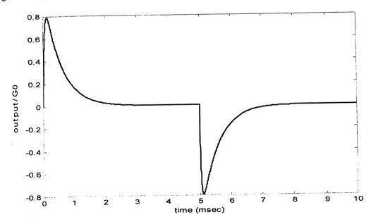
(c) The 5 msec rectangular pulses of a direct 200 bit /s signal will each be converted to the shape shown above. A run of positive/negative pulses will become a single positive/negative 'blip' at the start and then a zero signal. Hence simple thresholding cannot be used to recover the transmitted signal.
