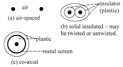
The maximum data rate over a cable circuit is proportional to its bandwidth, which in turn is inversely proportional to the product of the cable's shunt capacitance and its loop (series) resistance. The **air-spaced pair cable** has much lower capacitance per unit length, and hence higher bandwidth, than the solid-insulated pair cable. Such cables (strung between 'telegraph poles') were the original choice for long-distance telegraphs (and then telephones).
