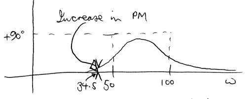
Hence system remains stable and phase margin is increased by  $\angle k(j34.5) \approx 13-7^{\circ}$ .
