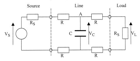
The *Loop resistance* of the cable  $R_{loop} = 4R$ .
