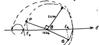
.', Points P, Q correspond to strain gauges, and gauges read normal strains Ep, Eq.
