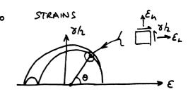
SO: strain gauges at 45° to hoop, longit. dirns correspond to points at 90° from hoop, longit points on Mohr's circle
