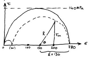
... Torque at point  $T = (2\pi r^2 t) T_m = 2\pi (400 mm)^2 (5 mm) \times 120 N/mm^2$ of yielding T = 2AetT ENGINEERING TRIPOS, PART IB, JUNE 2002
