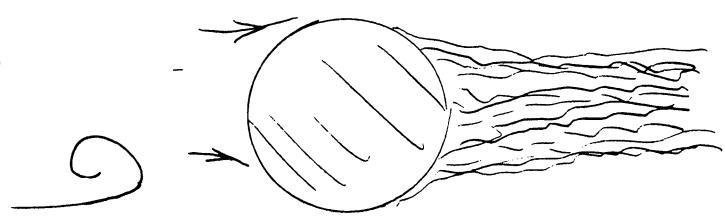
(c) frequency  $\omega = f(V, d, \mu)$  (viscosity not important)
