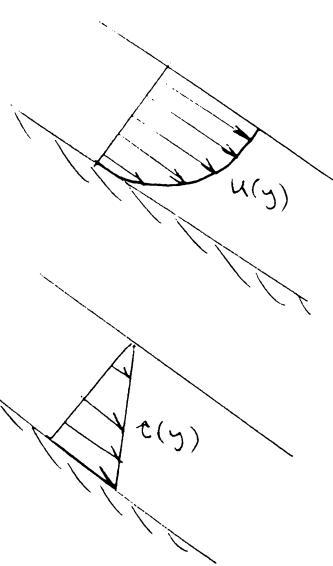
(5) (a) At 1 and 2 there is uniform horizontal motion. The vertical forces acting on a fluid element must therefore sum to zero (no vertical acceleration). Thus gravitational and pressure forces balance - i.e. we have a hydrostatic force balance.
