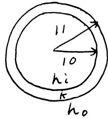
$$Q = h_i (\Delta T_{\text{OUTER}}) 2\pi r_i$$
