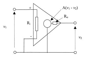
Summing currents at the output, we can find the gain,  $v_2/v_1$
