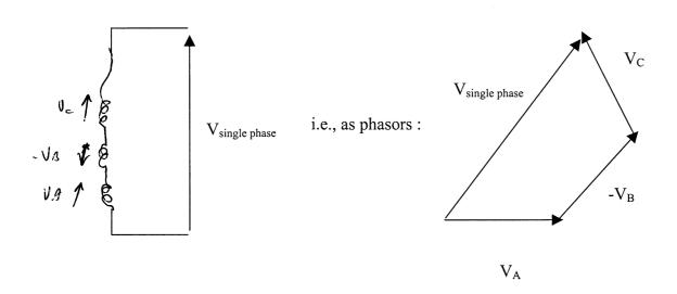
Geometrically,  $V_{single\ phase}=2V_A$   $\textit{Alternatively}, \ if \ we \ write \ V_A=V, \ V_B=Ve^{-j2\pi/3}, \ V_C=Ve^{j2\pi/3}$  We can combine these to find  $V_A$  -  $V_B+V_C=V(1+j\sqrt{3})=2V$   $\text{Therefore, the power is reduced from } 3V_{ph}I_{max} \ \text{to } 2V_{ph}I_{max}, \ \text{which is a factor of } 1/3.$
