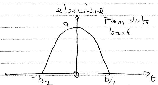
This is time shifted (by  $t_s/2$ ) compared with the half-sine pulse in the data book. A time shift however is equivalent to a phase shift of  $e^{-j\omega b/2}$  in the frequency domain which has no effect on the magnitude of the frequency response  $|H(f)|$ .
