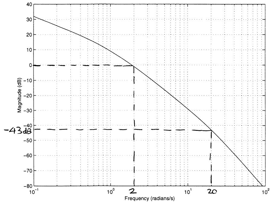
$$\begin{aligned} GM &= -43 + 10 \cdot 6 \\ &= -32.6 \\ \text{i.e., } &\underline{\underline{33 \text{ dB}}} \end{aligned}$$
