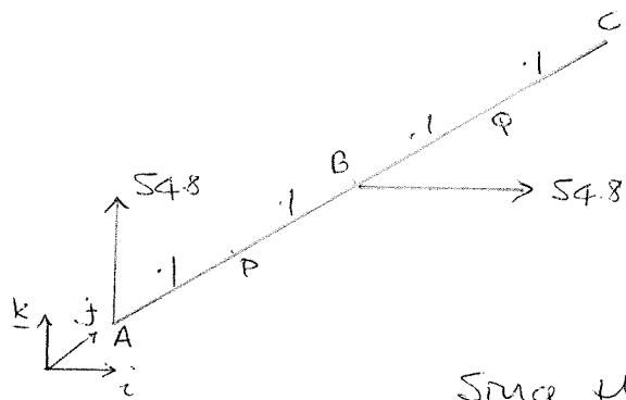
By inspection, taking moments about A the balancing mass at C must generate a force to balance the moment produced by 54.8 acting at B.
