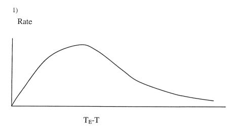
The rate is zero at  $T_E$  and at 0K so we get a peak at an intermediate temperature. This corresponds to a minimum in the time needed to effect a transformation, hence the nose in the curves at a temperature a bit below the transformation temperature.
