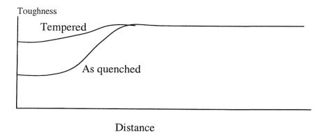
Decreased hardness causes an increase in fracture toughness.
