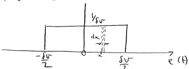
The power ( $\text{re}, \text{volt}^2$ ) of a noise value of amplitude  $x$  is  $x^2$
