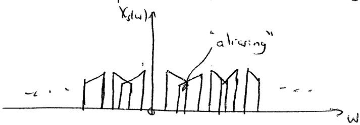
To eliminate aliasing distortion,  $f_s$  must be at least twice the maximum frequency present in the input signal.
