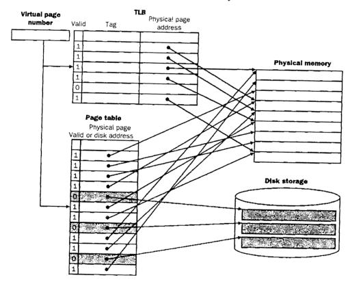
(b) In both cases there is a small, fast, expensive memory which stores a dynamic subset of a large, slow, cheap memory. With careful tuning, the combined system approaches the speed performance of the fast memory while offering the capacity of the large memory.
