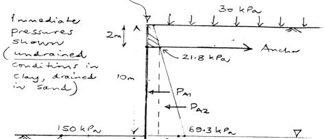
Sand  $8 = 18 \, \text{kN/m}^3$   $\phi' = 30^\circ$
