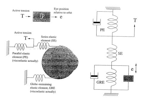
(b) The effect of inertia is negligible because the system is heavily over-damped, dominated by a low-frequency pole. Experimentally, the inertia has to be increased by a factor of around 100 before there is any sign of transient oscillation in a saccade. The visual effect of frequencies beyond some 30 Hz is negligible, because of the low-pass filtering exerted by the early stages of visual processing.
