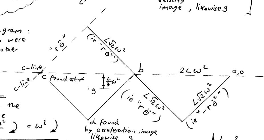
(c) For driving torque use the method of instantaneous power. Use d'Alembert's principle to deal with inertia forces.
