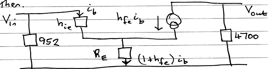
$$\text{Gain} = \frac{V_{out}}{V_{in}} = \frac{-h_{fe} i_b \cdot 4700}{h_{je} i_b + R_E (1+h_{fe}) i_b} = -\frac{4700 h_{fe}}{h_{je} + (h_{fe} + 1) R_E}$$
