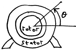
A rotating magnetic field is established in the air gap by the balanced three phase coils wound on the stator.
