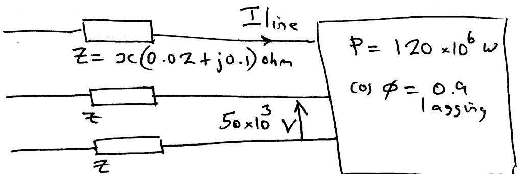
The line current per phase  $I_{\text{line}} = \frac{1}{\sqrt{3}} \frac{P}{\cos \phi} V$
