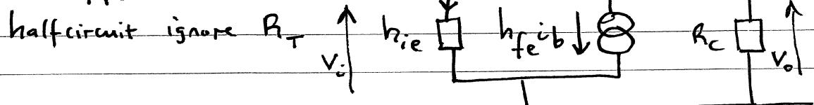
$$A_{\text{diff}} = \frac{V_o}{V_i} = \frac{-h_{fe} i_b R_c}{h_{ie} i_b} = -\frac{h_{fe} R_c}{h_{ie}}$$
