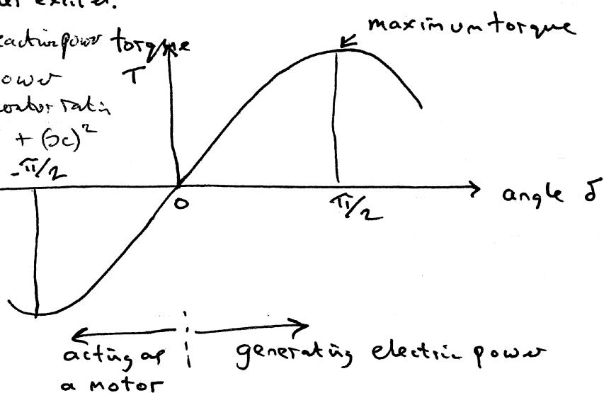
The point  $\delta = 0$  is special because no mechanical power is transferred
