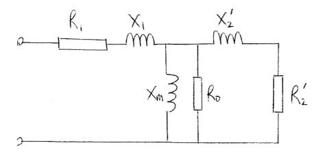
When rotor rotates at speed  $\omega_r$ , define slip as  $s = (\omega_s - \omega_r)/\omega_s$
