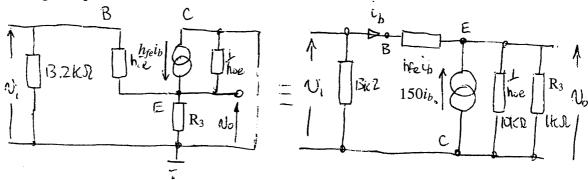
Note that output is taken from the emitter, and the collector is grounded for the SS analysis. (Common errors were to overlook the ground connection for the collector in the SSEC for this configuration, and to show  $v_o$  taken from the collector – should be the emitter – or to ignore the effect of  $1/h_{oe}$ )
