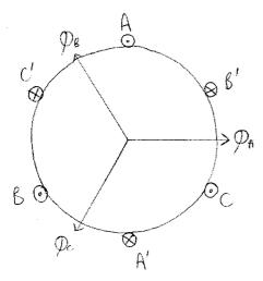
The flux axis of phase A is  $0^0$ , B is  $120^0$  and C is  $240^0$ . When each phase is excited in turn, the field distribution rotates. A balanced 3 phase supply in effect causes each phase to be excited in turn, hence producing a rotating magnetic field.
