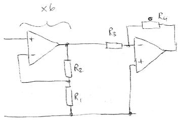
Let  $R_2 = 5R_1$  so gain = 6 With op-amps of ideal (infinite) gain, the input resistance of this stage will be infinite. In practice it will be many  $M\Omega$ .
