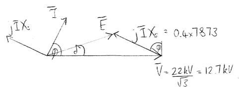
$$V_1 = 22.10^3 / \sqrt{3} = 12.7 \text{ kV}$$
