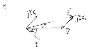
c/ 60% rated MVA =  $0.6 \times 500 = 300$ MVA, power factor = 0.6 leading
