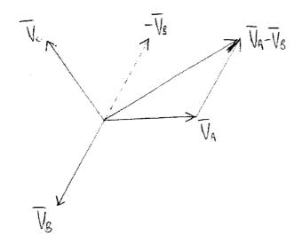
$V_{line} = V_1 - V_2 = |V_l| = 2V_1 cos \\ 30 = \sqrt{3.} V_1 \ \ in \ magnitude. \label{eq:Vline}$
