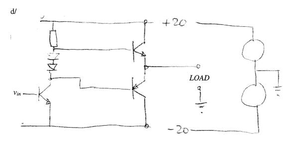
(Common errors were to use an NPN device rather than a PNP device, or to connect the PNP with emitter to -20 V, or some other non-follower configuration)
