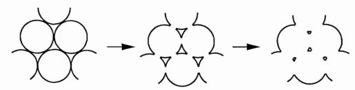
At a microscopic level, atoms diffuse from the grain boundaries between particles into the pores. Fine particles sinter much faster than coarse particles since the have a larger energy per unit volume, and hence a larger driving force for sintering, and the distances involved in diffusion are shorter.
