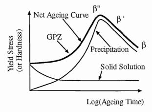
Solid solution hardening decreases as precipitates form from the supersaturated matrix.
