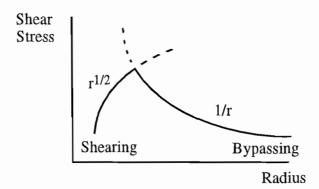
The maximum hardness usually coincides with the formation of the  $\beta$ ' phase. Overaging occurs when the incoherent precipitates coarsen further, and their separation increases. This can be reversed by heating the alloy above the  $\alpha/(\alpha+\beta)$  solvus line to re-dissolve the  $\beta$  phase and the second heat treatment repeated.
