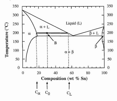
(d) 60 wt % Sn and 40 wt % Pb is the eutectic composition for this system, which has the lowest possible melting point ( $\approx 185^{\circ}$ C)/highest fluidity for a Sn-Pb alloy. This alloy is particularly useful as a solder (since it is easily melted) for electronic applications, where it is desirable to minimise the heat input into individual devices.
