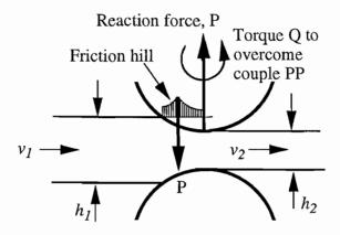
(c) Only one curve is required (note asymmetry of friction hill);
