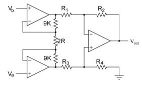
Connect two instances of Fig. 4 at each input of Fig. 3, as shown. The resultant circuit is the widely used Instrumentation Amplifier. Because of the symmetry of the circuit there is no need for the two resistors R to be grounded. This reduces the common mode gain. The extra stages:
