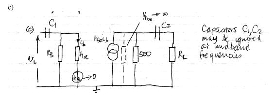
The Thévenin equivalent of the output circuit is a voltage source of  $500 \times h_{fe} i_b$  in series with a Thévenin resistance of  $500 \Omega$ . Capacitors C<sub>1</sub> and C<sub>2</sub> may be ignored at mid-band. Hence the optimum load for maximum power transfer is  $R_L = 500$  ohm.
