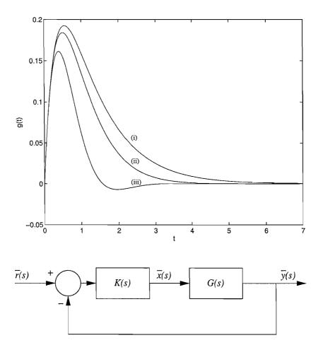
therefore increasing  $k_1$  will increase the bandwidth (the system will be able to follow signals that change more rapidly) and increasing  $k_2$  leads to an increased damping, therefore to a more stable system, where oscillations due to a disturbance will die down more quickly.  $k_1$  . Leads damping (Lighty).
