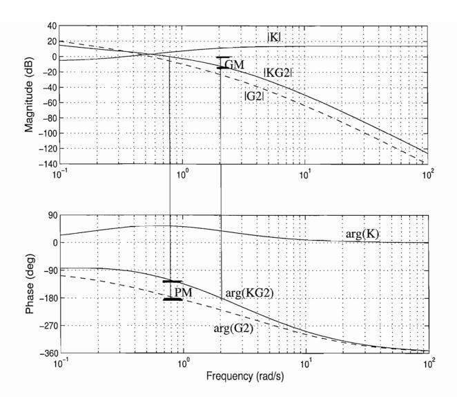
2 (a) If we input into the open-loop system harmonic functions of different frequencies, then the response will oscillate on the same frequency. Once the transients have died down, the measured ratio of the output to input amplitudes will give us the magnitude of the transfer function, while the measured phase difference between input and output is the argument of the transfer function for the corresponding frequency.
