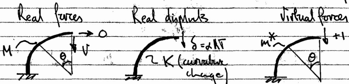
$$\text{Real } K = \frac{EI}{R}, \text{ where } VR \sin \theta = M \text{ (bending moment)}$$
