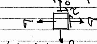
$$\sigma = \frac{M \cdot b}{I} ; \gamma = \frac{T}{\frac{I}{2 \cdot b^2}} \leftarrow \begin{matrix} \text{wall} \\ \text{thickness} \end{matrix}$$
