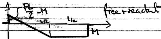
$$\left| \frac{FL}{2} - M \right| \leq M_p, \quad M \leq M_p \Rightarrow F_{\max} = \underline{\underline{4M_p/L}}$$
