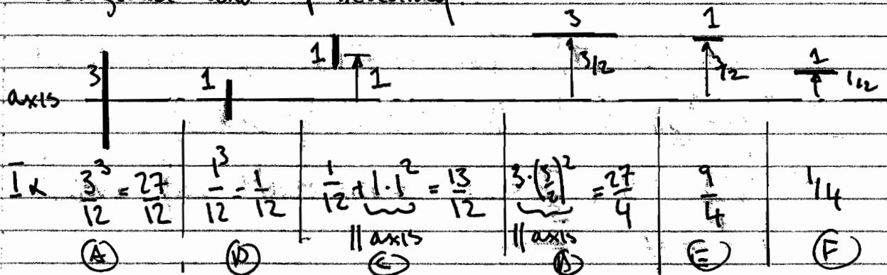
$$\text{For square section } I \propto \left[ 2 \times (A) + 2 \times (D) \right] = 2 \left[ \frac{27}{12} + \frac{27}{4} \right] = 54/3$$
